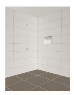
STEP 5 Apply tile to shower tray, walls, and bathroom. Adhere glazing channel to tiled tray and walls.
